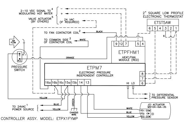
MINIMUM 40 VA. UP TO 20 VA AVAILABLE FOR HOT WATER ACTUATOR (BY OTHERS). REFER TO FAN WIRING DIAGRAM FOR TRANSFORMER AND RELAY WIRING, AND OTHER HIGH VOLTAGE WIRING.
