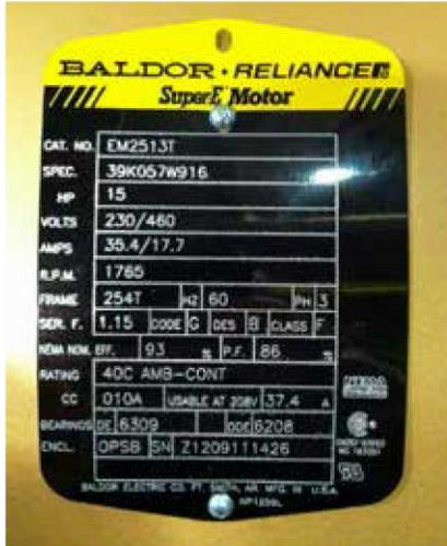
FIGURE 62 - TYPICAL MOTOR DATA/NAME PLATE
