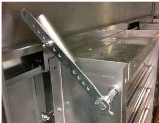
**FIGURE 51 - COUNTERBALANCE UNLOCKED FOR START-UP**
