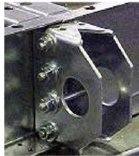
Baserail Lifting Lugs Assembled
