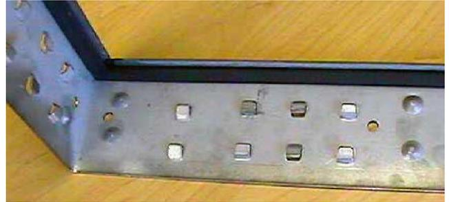
**FIGURE 114 - CORRECT USE OF KNOCKOUTS**
