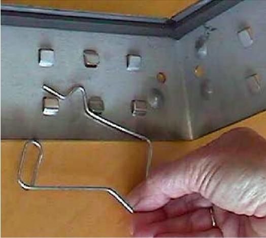
**FIGURE 112 - CORRECTLY INSTALLED LATCH PIN**
