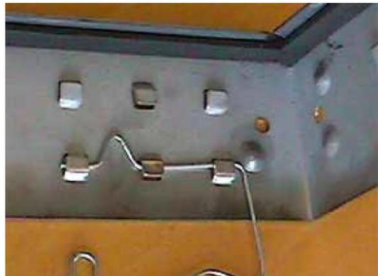
**FIGURE 109** - CORRECTLY INSTALLED LATCH PIN (P/N 026-35778-007)
