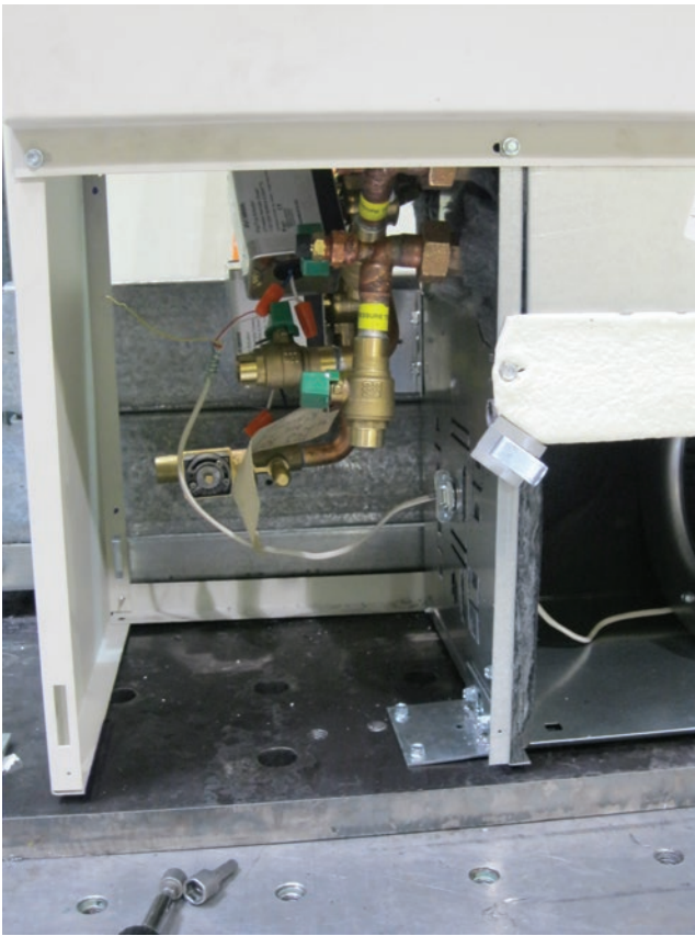
FIGURE 7 – FRONT CLIPS ATTACHED TO UNPAINTED SHEET-METAL FRAME.
