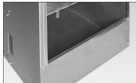
Positively sloped drain pan prevents standing water; lined with closed cell foam insulation for added moisture protection.
